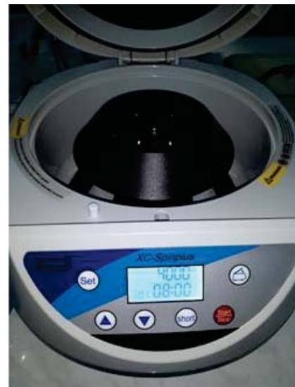
Figure 4. Programmable centrifuge, Rotor radius 100mm
