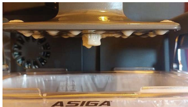
Figure 4. Group 4. Image during printing of the restoration
