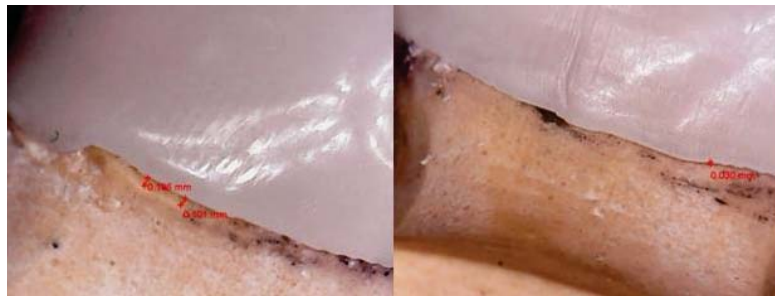
Figure 9. Microscopic evaluation of the cervical adaptation of the group 4, printed restoration. Spacing between the crowns margin and the limit of the marginal preparation
