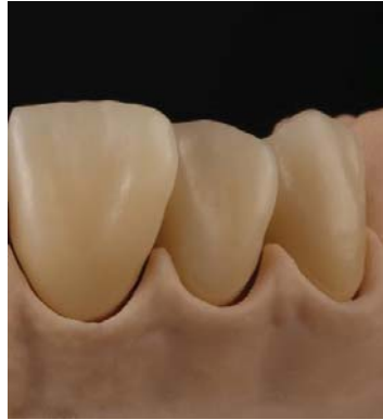
Figure 6. Three zirconia crowns after sintering process on the control model
