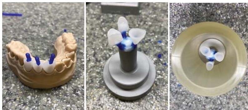
Figure 8. The attachment of rod wax on each milled wax crown; b. the attachment of rod wax on silicone pattern; c. the packaging cylinder
