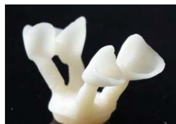
b. Figure 3b. Pressed ceramic coping
