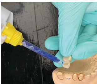
Figure 1. Layering of silicone on the inner surface of the samples of group 2
