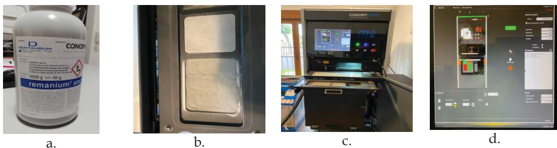
Figure 10. a. The used metal powder; b. Introducing the metal powder into the Concept Laser; c. Entering STL data in the Concept Laser; d. Programming for milling
