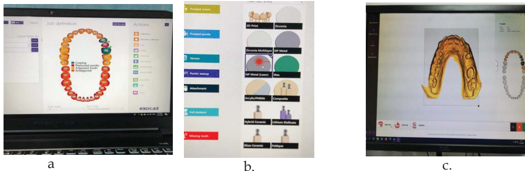
Figure 2. a. Completing the patient file, selecting abutments, neighbouring teeth and antagonists; b. Material type selection, in this case NP Metal (Laser); c. Scanning maxillary model
