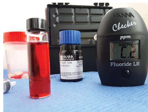
Figure 5. HI-729 Fluoride Low Range Handheld Colorimeter, Checker®HC device
