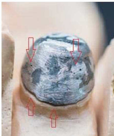
Figure 15. The defects on the metal infrastructure
