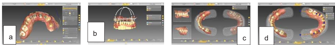
Figure 4. a. edit model stage; b. checking of the occlusion; c. aligning the cast and establishing the model axis; d. drawing the curves of both arches and establishing the position of each tooth
