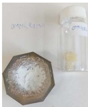
Figure 1. Streaming Potential Analysis of a Dental Composite: Powderization and Measurement Using the PCD Device
