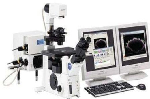
Figure 4. Laser scanning confocal microscope Olympus Fluoview FV1000 used for morphological evaluation of enamel specimens
