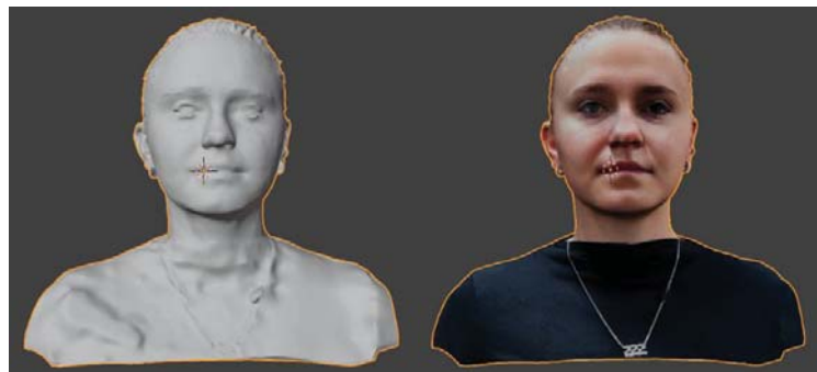
Figure 1. Geometry and color texture of Subject 1 obtained with LiDAR (Qlone Application).
