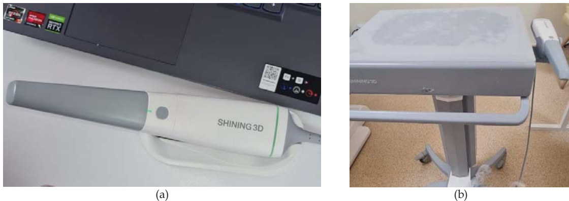
Figure 1. The Aoralscan 3 intraoral scanner (SHINING 3D). (a) Handpiece of the Aoralscan 3 intraoral scanner. (b) Mobile scanning unit with the attached Aoralscan 3 scanner
