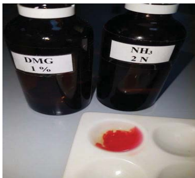
Figure 7. Fe 2+ ion identification reaction in the presence of dimethylglyoxime on the well plate
