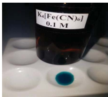
Figure 4. Identification reaction of Fe^{3+} ion in the presence of potassium ferrocyanide on the well plate
