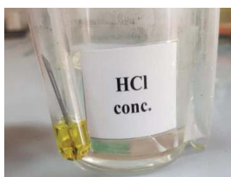
Figure 3. Solubilization of the collected sample in concentrated HCl (37%)
