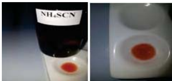
Figure 5. Identification reaction of Fe 3+ ion in the presence of ammonium sulfocyanide on the well plate
