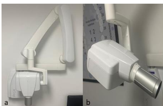
Figure 4. Extraoral radiographic device (Planmeca ProX) used for CBCT imaging. a) Frontal view showing the structural design and positioning arm; b) Lateral view illustrating the alignment and tube head orientation used during imaging of the samples
