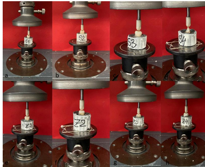
Figure 9. Positioning of samples from both groups - S (fiberglass-reinforced composite) and Z (zirconia-based) - in the universal testing machine prior to mechanical testing: a) S1, b) S2, c) S3, d) S4, e) Z1, f) Z2, g) Z3, h) Z4
