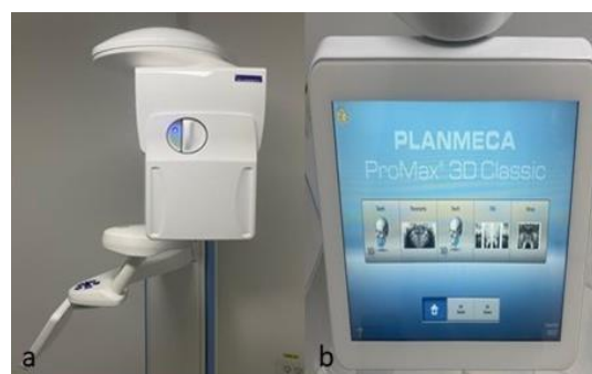
Figure 5. Cone-beam computed tomography (CBCT) system used for sample imaging: Planmeca ProMax 3D Classic. a) Lateral view illustrating the CBCT unit and patient positioning arm; b) Control display interface used for parameter adjustments and image acquisition monitoring
